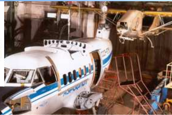
STATIC STRUCTURAL TESTS OF FUSELAGE
