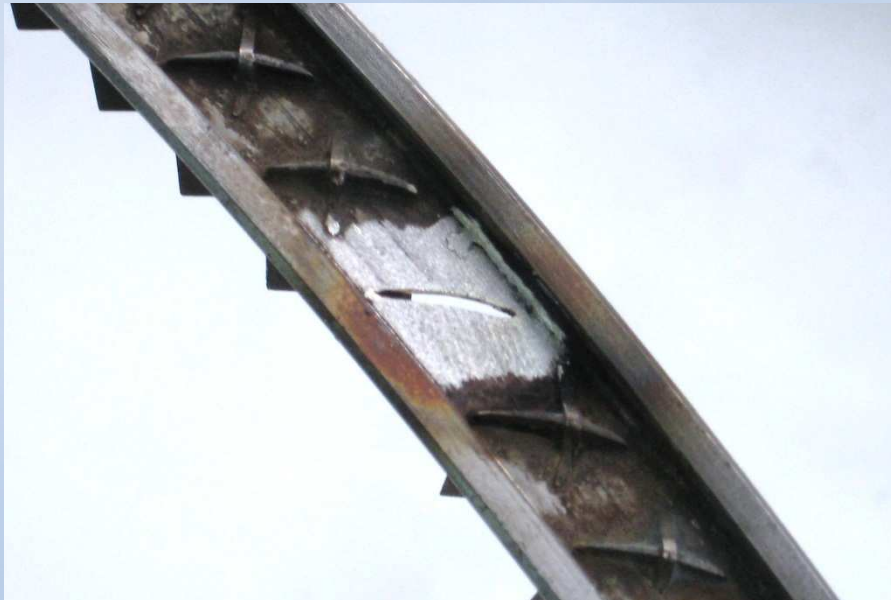
A. Debrazed non-conditional blade place
