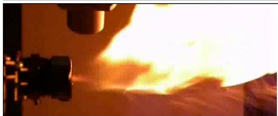
Photo of plasma assisted combustion of paraffin at different air flows: G=55 \text{ cm}^3/\text{s}^{-1} (top) and G=150 \text{ cm}^3/\text{s}^{-1} (bottom)
