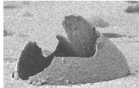
Scanning electron microscope image of a ruptured microcapsule Photo courtesy University of Illinois
