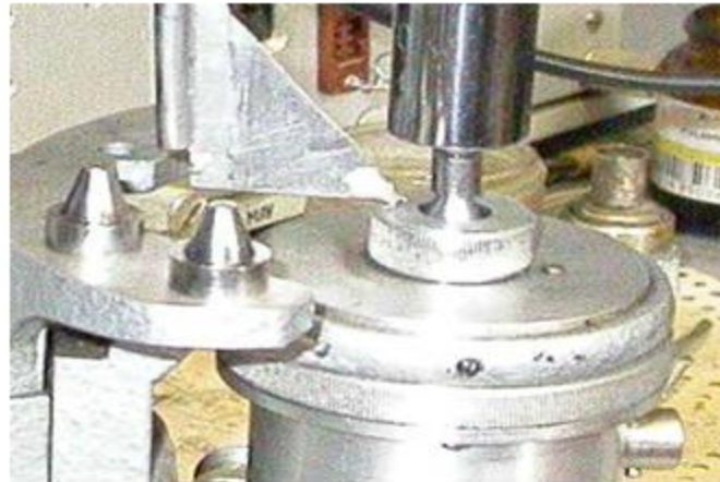
Low temperature dilatometer with the main parts manufactured from developed Invar alloy
