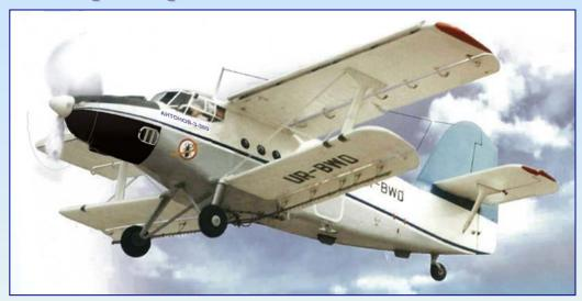
Aн-3-300 –developing of Aн-2 aircraft. Retooling AN-2 in AN-3-300 consist in change of piston engine on turboprop MC-14 by OAO «Motor-Sich» (Zaporozhe).
